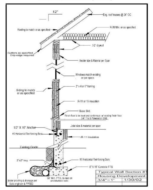
TYPICAL CONCRETE WALL SECTION (not to scale)
