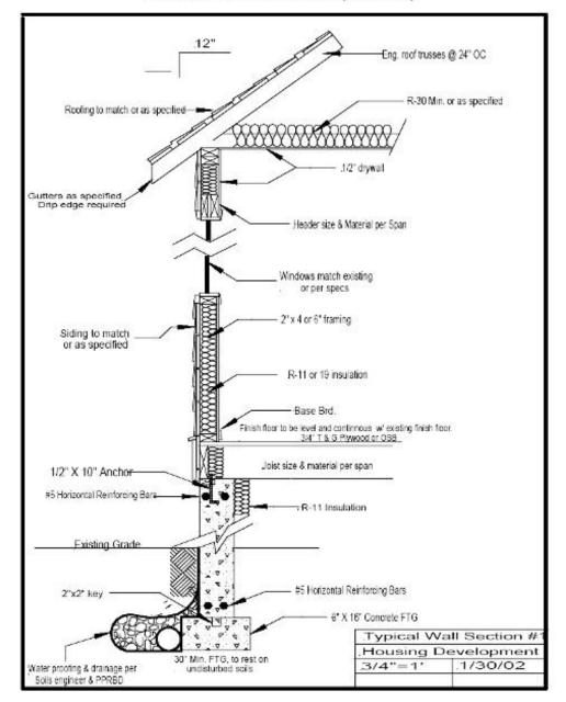
TYPICAL CONCRETE WALL SECTION (not to scale)
